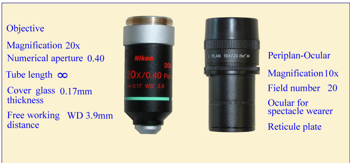
Figure 1-5. Objective (Example: Nikon CFI Achromat 20x P) and ocular (Example: Leica Periplan with reticule plate)
